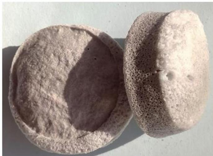
**Fig. 4. Samples of heat insulating coatings on the basis of hollow glass microspheres and foamed liquid glass.**
